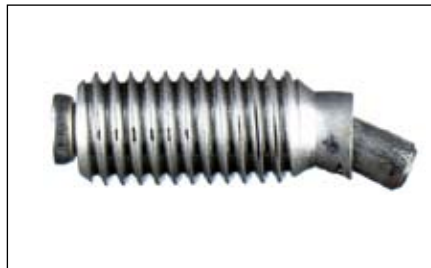
Plastic deformation of X-BT
