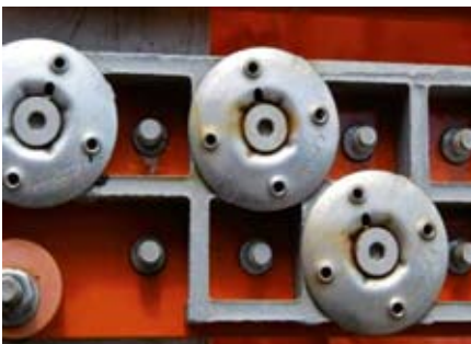
See water test rig with test specimens installed (X-BT with and without X-FCM grating discs).
