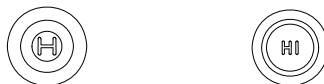
FIGURE 4—DEPICTION OF IDENTIFYING HEAD STAMP FOUND ON TOP OF THREADED STUDS: "H" FOUND ON CARBON STEEL STUDS AND "HI" FOUND ON STAINLESS STEEL STUDS
