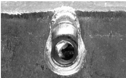
Plastic deformation of base steel
