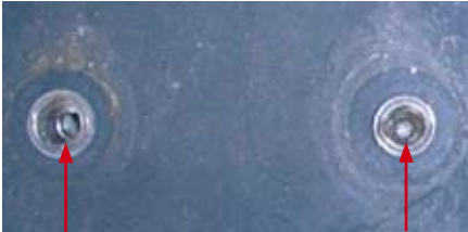
Drilled holes after 90 days salt spray test and after pull-out of the X-BT fasteners. These holes appear clean and no evidence of corrosion is visible.
