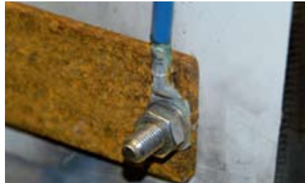
Test assembly X-BT with cable lug
