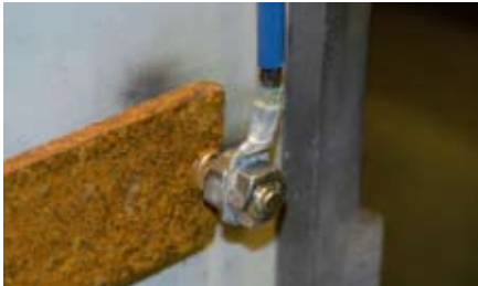
Test assembly X-BT with double nut
