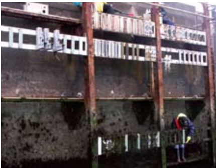
See water test rig with test specimens installed (X-BT with and without X-FCM grating discs).
