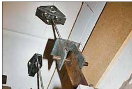
Centric and eccentric loading of the roller connector
