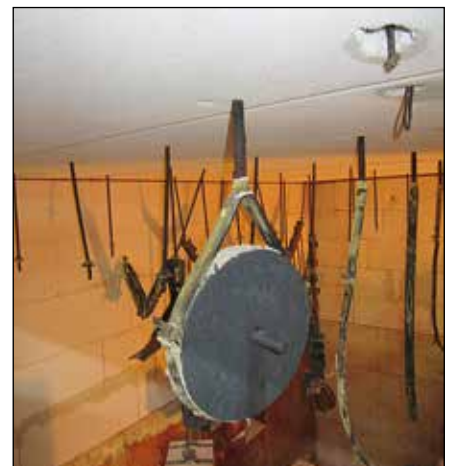
MP-MXI pipe ring with pipe dummy after the fire test
