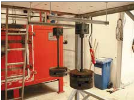
Fire test of MM-C channels with single load
