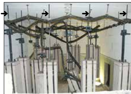
Multiple-span continuous beam with single loads, after the fire test → = Deformation measurement
