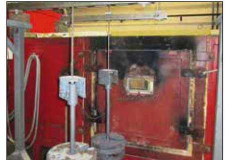
Suspended MQ installation channel with central single load before the fire test
