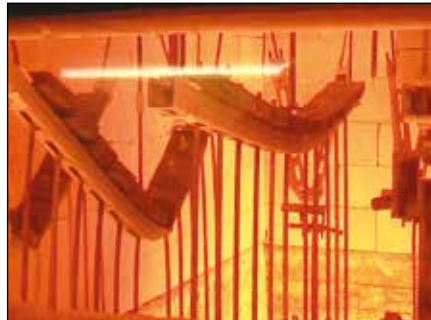
Significant deformation of the channels when exposed to fire, depending on the applied load and the duration of the fire
