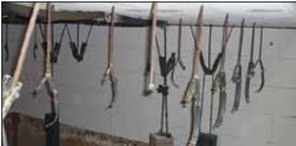
Pipe rings after the fire test, failure in the locking mechanism
