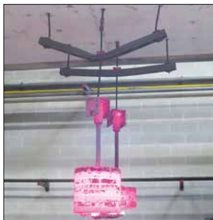
Suspended MQ installation channel with central single load. The central threaded rod is used for measuring the deformation
