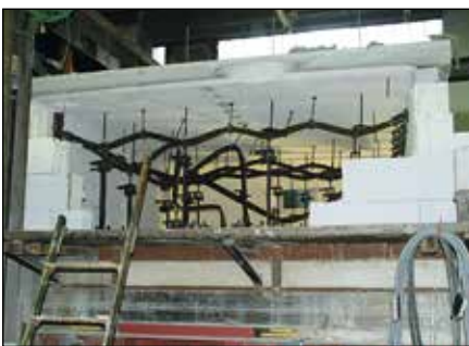
Multiple-span continuous beam systems with single loads, after the fire test
