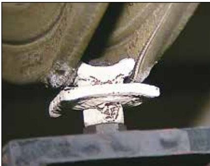
Deformation of MQA-B and channel MQ-41, shortly before failure
