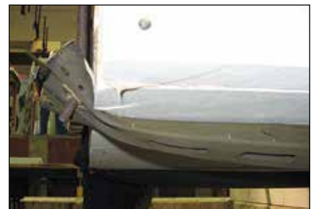
Severe deformation of the mounting channel in the corner area, the threaded rods are in contact with the duct, hardly any deformation of the mounting channel
