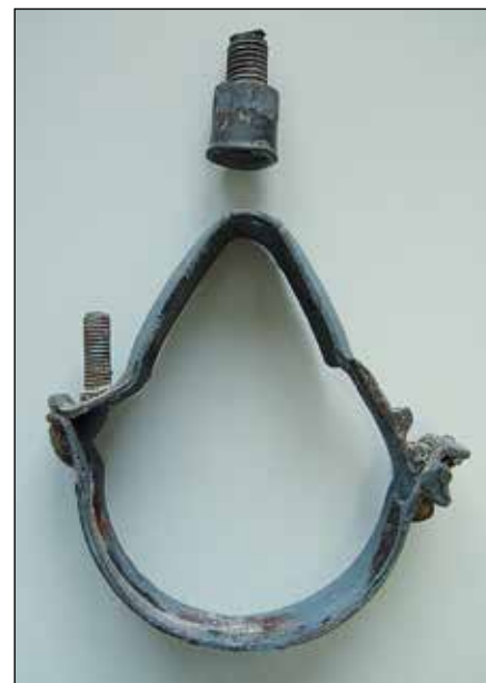
Pipe ring after the fire test, tearing of the connection boss
