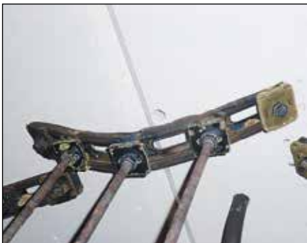
Directly-installed channel MQ-21, span 350 mm, 3 single loads
