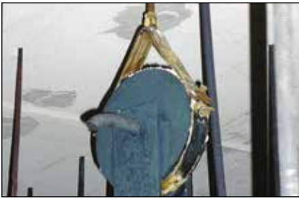
Pipe ring after the fire test, no failure, severe deformation in at the closing mechanism
