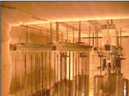
Suspended MQ installation channel with equal load immediately after the start of the fire test
