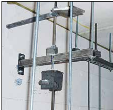
MQK bracket with central single load before the fire test
