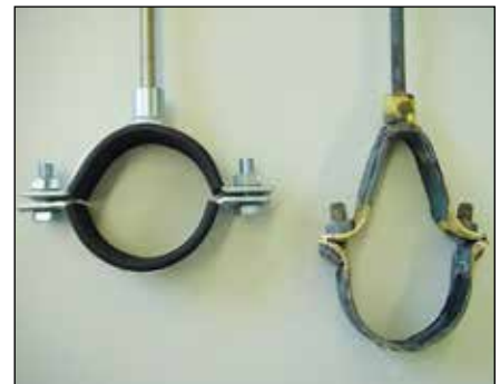
MP-MXI pipe ring before and after the fire test
