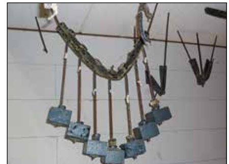
Suspended MM-C installation channel with multiple load after the fire test
