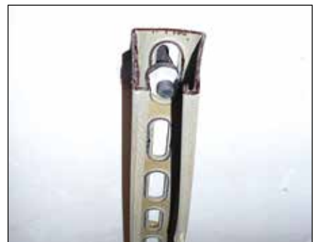
MM-C channel, with central single load, low partial deformation after failure of MM-S
