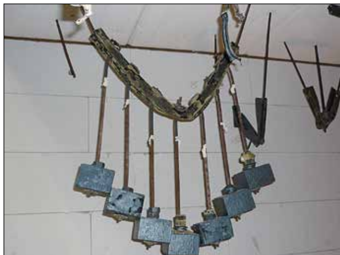
Suspended installation channels with multiple load after the fire test
