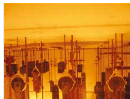
MP-MXI pipe rings, view inside the furnace after the end of the fire test
