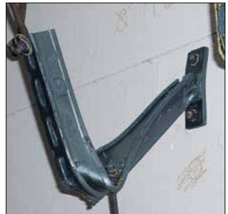
MM-B bracket with central single load after the fire test
