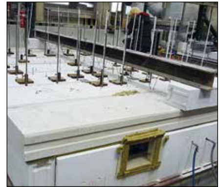
Furnace: Roof made of gas concrete ceiling sections, observation window at the front
