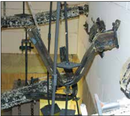
Bracket composed of MQ-41/3 channel, MQP-21-72 channel support and MQN channel connectors, suspended at one end, after the fire test
