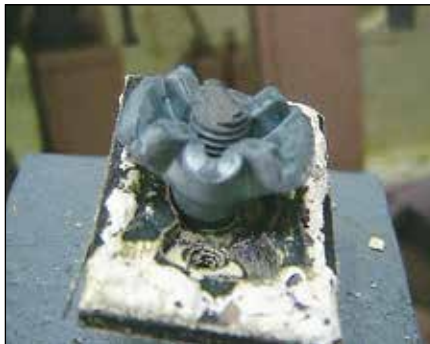
Extreme deformation of the MQA channel nut with cold-formed sheet metal nut
