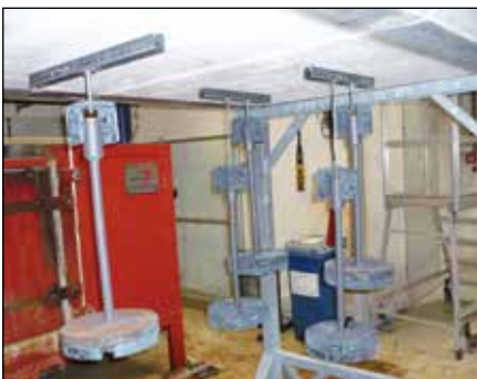
Preparation for fire test with MM-C-45
