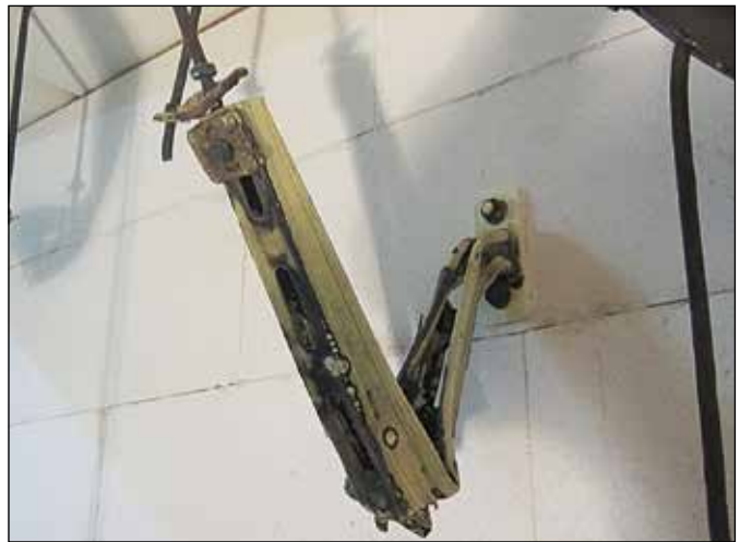
MQK bracket with central single load after the fire test
