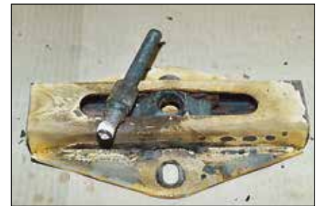
Mode of failure: threaded tubing pulled out of the carriage
